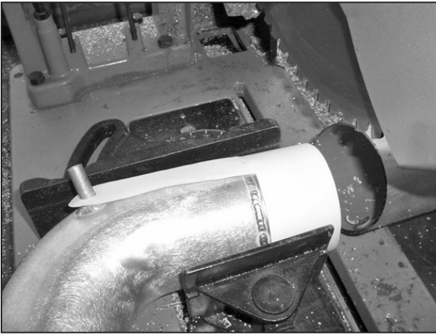
j. Saw the intake tube at the edge of the template.
