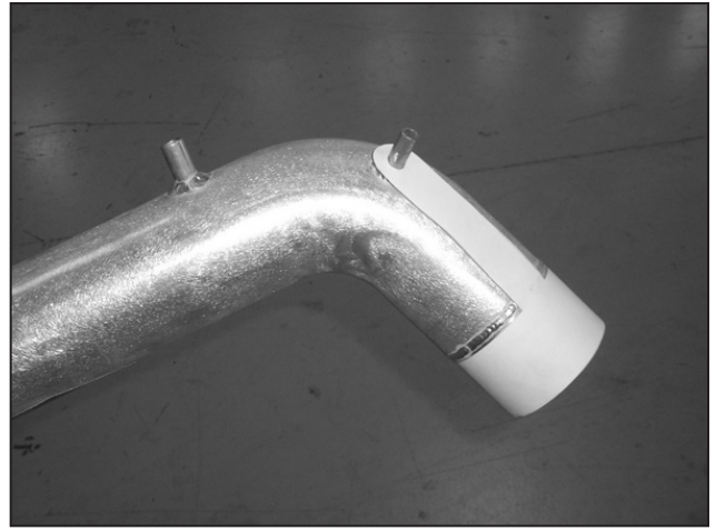
k. Once the intake tube is properly cut, it should look like this.
