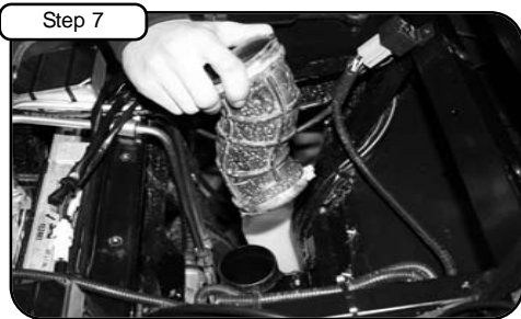
Remove OE intake tube out of Rhino.
