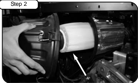
Step 2 To remove air-box cover, un-clip upper half of air box with OE air filter and remove.
