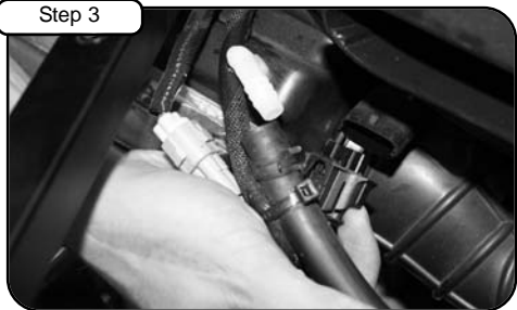
Step 3 Disconnect crankcase line and temp sensor from air box. Loosen clamp with 1/4" nut driver or flat head screwdriver.
