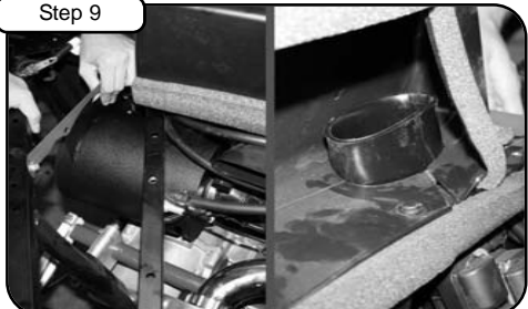
Step 9 To install housing into RZR, guide into factory intake tube and position to bracket. Use factory screws from step 4. Guide coupler to factory position. Do not tighten.
