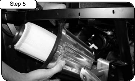
Step 5 Remove air box from intake tube.
