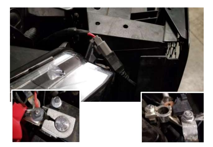
36. Before installing the aFe Scorpion grille, install the supplied power harness. The Red wire goes on the positive battery terminal (+) and the black wire goes on the negative battery terminal (-). You will need to mount the switch inside the cab or to an available prewired switch. Use the (15) supplied 8" cable ties to secure the wiring loom to the vehicle.
