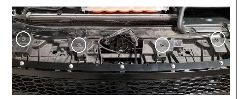
39. Center the grille assembly and install the four (4) factory screws removed in Step 4. Tighten to factory specifications.
