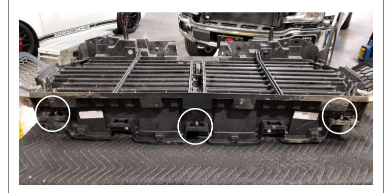
32. Attach the active shutter grille to the aFe Scorpion grille. At the bottom of the aFe Scorpion grille assembly, install three (3) supplied 3/16" x 1" SS fender washers (black) and three (3) #10-32 nylon lock nuts. Do not tighten.
