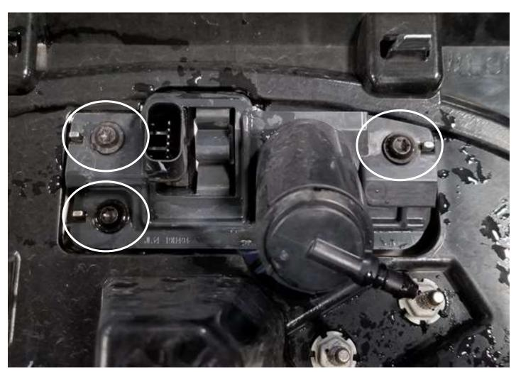
16. Remove the FFC and the FFC washer assembly from the factory grille.
