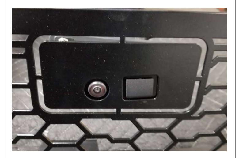
22. Reinstall the FFC mounting bracket onto the aFe Scorpion grille using the hardware removed in Step 19. Before tightening, make sure to center the camera and the washer.
