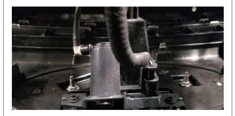
12. Disconnect the electrical connector from the FFC and the FFC washer water hose.
