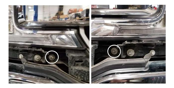
8. Remove the one (1) bolt located on each side of the grille. Save for reinstallation.
