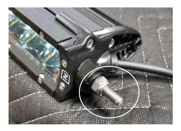
23. Remove and discard the two (2) nuts from the supplied 20" single row LED light.
