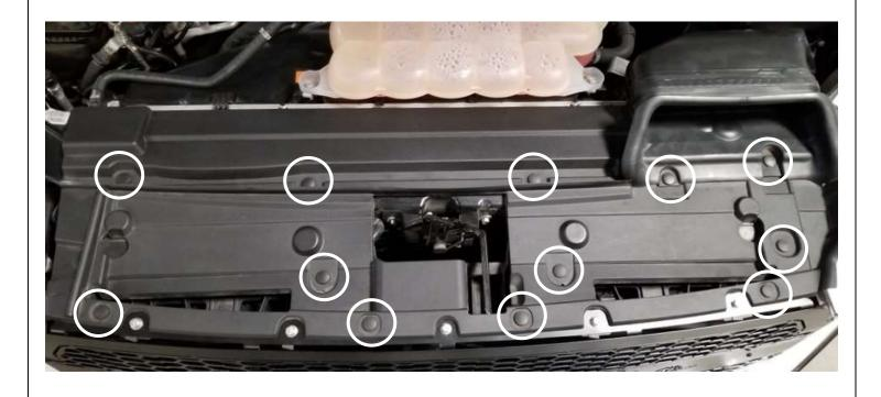
45. Install the plastic shroud and the (12) plastic clips removed in Step 2.
