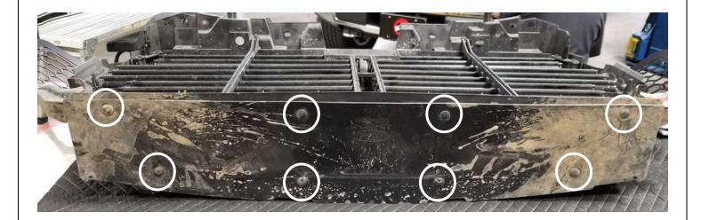
35. Reinstall the eight (8) push pins that attach the plastic lower shroud.
