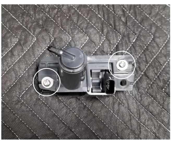
20. Install the FFC assembly to the FFC mounting bracket with the two (2) supplied #10-32 x 5/8" button head screws, two (2) supplied #10 flat washers, and two (2) supplied #10-32 nylon lock nuts.
