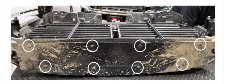
11. Remove the eight (8) push pins and remove the plastic lower shroud.
