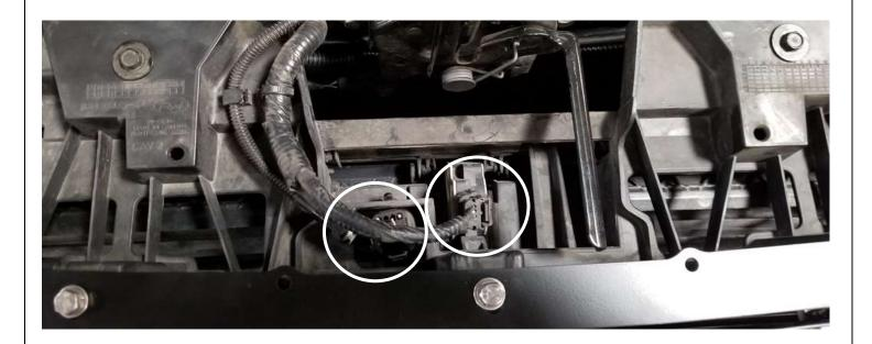
44. Reconnect the wiring connectors and the FFC washer hose connection.
