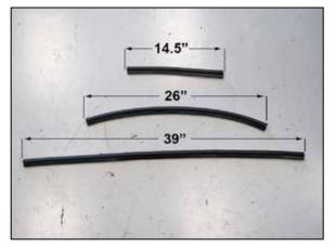
9. Cut the provided edge trim into three sections, one section will be 39" long, one section will be 26" long and the final section will be 14.5" long.
