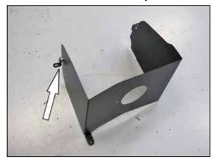
8. Install the heat shield mounting bracket (070066) onto the heat shield using the provided spacer and hardware.
