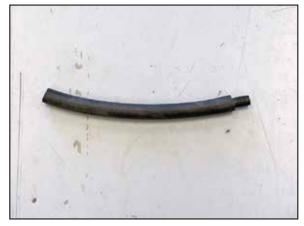
19. Install the hose mender into the provided crank case vent hose as shown.
