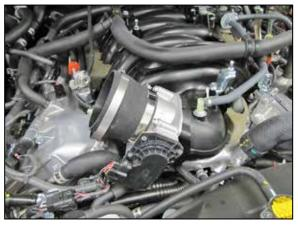
14. Install the coupling hose (08050) onto the throttle body and secure with the provided hose clamp.
