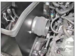
15. Install the hump coupler (08418) onto the filter adapter and secure with the provided hose clamp.
