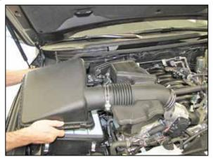
6. Release the four retaining clips securing the upper air box and then remove the upper air box and intake tube assembly from the vehicle.
