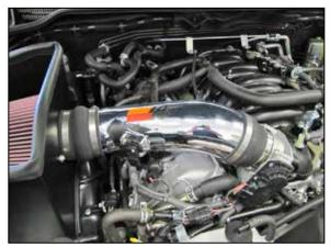
20. Install the K&N<sup>®</sup> intake tube into the hump coupler at the heat shield and then into the coupler at the throttle body, adjust the tube for best fit and
