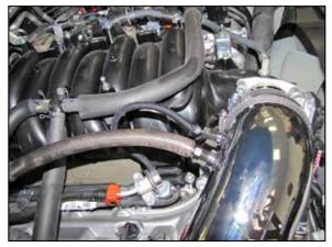
21. Install the crank case hose assembly into the factory crank case vent, Then connect the crank case vent hose and the fuel pressure hose to the fittings installed into the K&N<sup>®</sup> intake tube.
