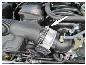
4. Loosen the hose clamp which secures the intake tube to the throttle body.
