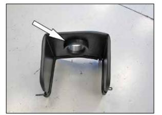
11. Install the filter adapter onto the heat shield and secure with the provided hardware.
