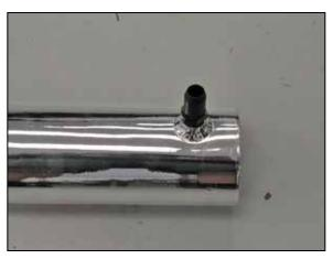
17. Install the provided vent fitting into the K&N® intake tube as shown.
