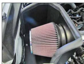
21. Install the K&N® air filter onto the filter adapter and secure with the provided hose clamp.
