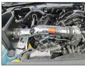
18. Install the intake tube into the coupling hose at the throttle body and then into the coupling at the filter adapter. Adjust the tube for best fit and then secure with the provided hose clamps.
