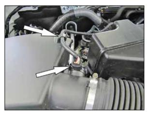
5. Disconnect the mass air sensor electrical connection and unhook the harness from the air filter housing.
