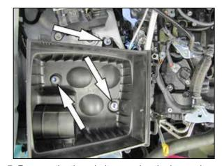
7. Remove the three bolts securing the lower air filter housing to the inner fender and then remove the lower air filter housing from the vehicle.
