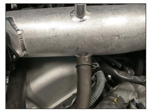
27. Connect the crank case vent hose to the K&N<sup>®</sup> intake tube and secure with the stock hose clamp.
