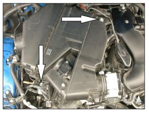
8. Remove the two air box mounting bolts shown and loosen the hose clamp at the throttle body.
