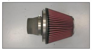
25. Install the provided silicone hose (08724) onto the K&N<sup>®</sup> filter assembly and secure with the provided hose clamp.
