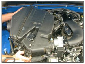
9. Lift up and remove the air box assembly from the engine.
