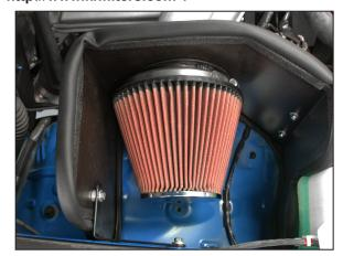
26. Install the K&N® filter assembly onto the K&N® intake tube and secure with the provided hose clamp.
