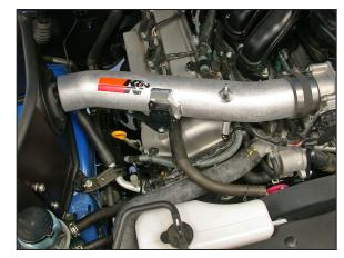
23. Install the intake tube into the silicone hose at the throttle body and align the mounting bracket with the threaded boss on the valve cover, then secure with the provided hardware and hose clamp.
