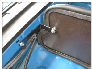
15. Secure the heat shield to the inner fender with the large "L" bracket as shown.
