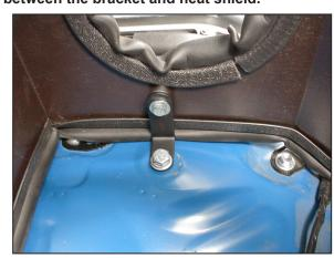
16. Secure the bottom of the heat shield to the inner fender with the small "L" bracket.
