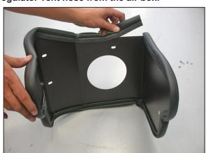
10. Install the long edge trim around the perimeter of the heat shield as shown.
