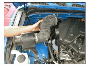
7. Loosen the hose clamp which secures the intake tube to the stock air filter housing and then remove the intake tube and resonator assembly.
