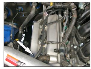
28. Install the provided vent hose onto the fuel pressure regulator and then onto the K&N<sup>®</sup> intake tube as shown.
