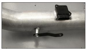
21. Install the tube mounting bracket (26545) onto the  $K\&N^{\otimes}$  intake tube as shown.
