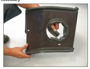
11. Install the short edge trim to the inside of the intake tube pass trough hole as shown.
