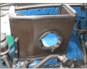
14. Install the heat shield into the vehicle and secure to the power steering reservoir with the bolt removed in step #13.
