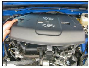
3. Lift up and remove the engine cover.
