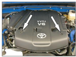
2. Loosen the two nuts that secure the engine cover.
