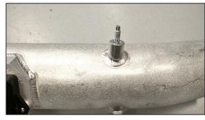
20. Install the engine cover mounting stud into the  $K\&N^{\otimes}$  intake tube as shown.
