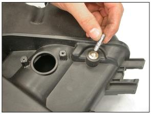
19. Remove the engine cover mounting stud from the factory air box.
