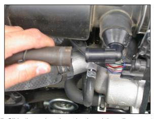
5. Slide the spring clamp back and then disconnect the crank case ventilation hose from the fitting on the factory air box.
