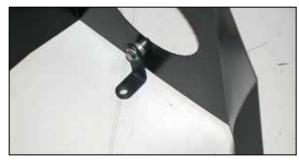
9. Install the small heat shield mounting bracket (070812) with the provided spacer onto the heat shield as shown.
