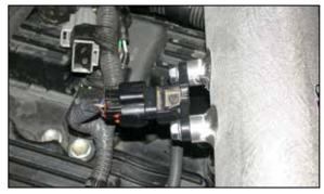
22. Install the pressure sensor onto the K&N<sup>®</sup> intake tube using the bolts removed in step #3.
