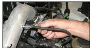
20. Install the provided vacuum hose onto the fuel pressure regulator and then onto the K&N $^{\odot}$  intake tube as shown.
