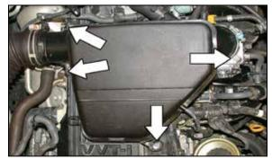
4. Remove the three bolts that secure the intake plenum to the engine and loosen the throttle body hose clamp.
