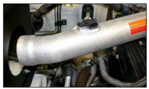
19. Secure the K&N<sup>®</sup> intake tube to the tube mounting bracket with the provided hardware and then tighten the hose clamp at the throttle body.
