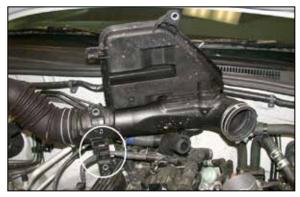
6. Disconnect the wire harness-retaining clip shown from the intake plenum.
