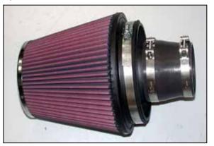
24. Install the provided silicone hose (084055) onto the K&N<sup>®</sup> air filter and secure with the provided hose clamp as shown.
