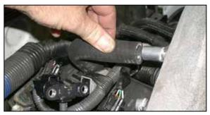
Install the provided crank case vent hose onto the valve cover port and then onto the K&N<sup>®</sup> intake tube and secure with the provided hose clamps.
