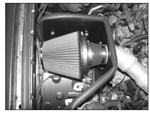
22. Install the air filter assembly onto the  $K\&N^{\textcircled{o}}$  intake as shown and secure with the provided hose clamp.
