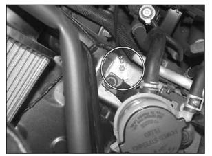
24. Using the bolt that was removed in the previous step, connect the ground strap to wheel well as shown.
