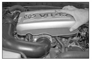
2. Loosen the two nuts that secure the throttle body cover, then remove the throttle body cover
