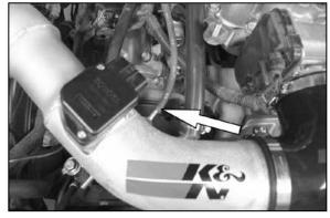
18. Connect the factory fuel pressure vent hose onto the  $K\&N^{\otimes}$  intake tube as shown.
