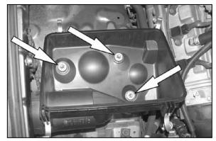
6. Remove the air box lid and filter to gain access to the three bolts that retain the air box to vehicle.
