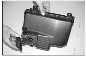
14. Remove the two screws that secure the mass air sensor to the air box lid, then remove the mass air sensor as shown.
