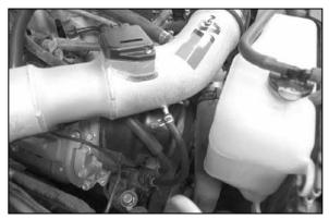
19. Connect the factory power steering pressure switch vent hose onto the K&N $^{\mbox{\tiny \ensuremath{\$}}}$  intake tube as shown.
