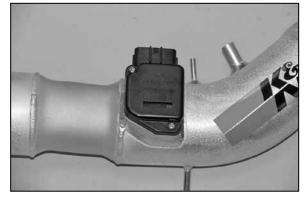
15. Install the mass air sensor into the  $K\&N^{\otimes}$  intake tube and secure with the provided bolts as shown.
