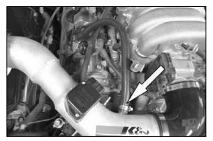
17. Remove the factory crank case vent hose from valve cover and then install the supplied vent hose onto the valve cover and K&N<sup>®</sup> intake tube and secure with the supplied hose clamp as shown.
