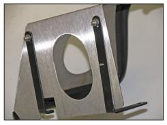
14. Install the provided "L" bracket #010054 onto the heat shield so that the other end of the bracket rests on the mounting tab on the strut tower as shown.
