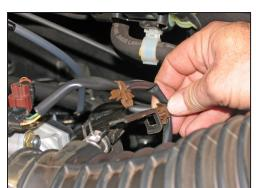
4. Unhook the wiring harness retaining clips as shown
