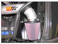
22. Install the K&N® air filter onto the intake tube as shown, and secure with the provided hose clamp.
