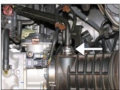
5. Using a pair of pliers, release the crankcase vent tube clamp and then disconnect the crankcase vent tube from the intake tube.
