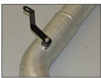
19. Install the tube mount bracket #010107 onto the K&N® intake tube as shown.
