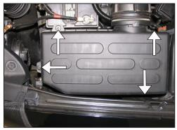
7. Loosen the four airbox lid retaining bolts shown.
