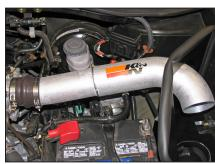
20. Install the K&N® intake tube into the silicone hose at the throttle body so that the mounting bracket rests on the heat shield mounting bracket and the mounting tab on the strut tower. Secure the mounting bracket to the heat shield bracket and mounting tab with the provided hardware and tighten the hose clamp at the throttle body.
