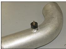
18. Install the provided rubber mounted stud onto the K&N® intake tube as shown.
