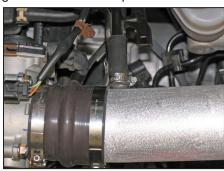
21. Install the provided silicone vent hose onto the K&N intake tube and then install the crank case vent tube into the silicone hose as shown. Secure the vent hose to the K&N® intake tube with the provided hose clamp as shown.
