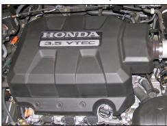
23. Reinstall the engine cover and secure in place with the three 1/4 turn fasteners.
