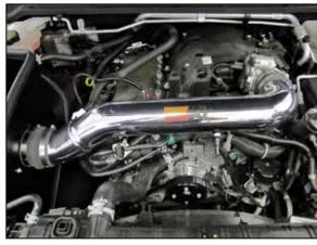
18. Install the intake tube assembly into the coupler at the filter adapter and then into the coupler on the throttle body. Adjust the tube for best fit and secure with the provided hose clamps.
