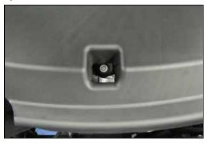
4. Remove the front center bolt securing the intake plenum to the engine and remove the intake plenum from the vehicle.
