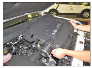
8. Lift up and remove the intake plenum from the engine.
