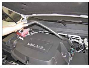
3. Disconnect the crank case vent hose from the intake plenum and then disconnect it from fitting on the valve cover and then remove it from the vehicle.
