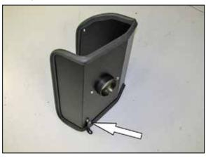
12. Install the provided heat shield mounting bracket (070015) onto the heat shield as shown using the provided hardware.
