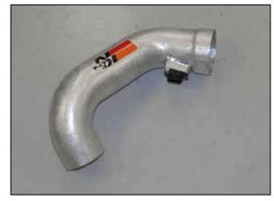
19. Install the mass air sensor into the  $K\&N^{\mbox{\scriptsize @}}$  intake tube and secure with the provided hardware.
