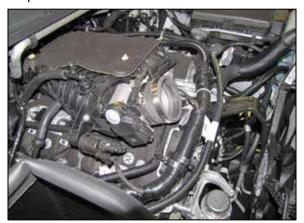
17. Install the provided step coupler (08186) onto the throttle body and secure with the provided hose clamp.
