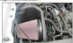
11. Install the filter assembly into the heat shield filter top first, then rotate the filter and pass the adapter through the hole in the heat shield. Secure the filter adapter to the heat shield using the provided hardware.
