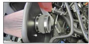
13. Install the provided hump hose (08699) onto the filter adapter and secure with the provided hose
