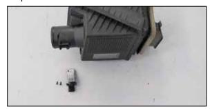
14. Remove the two screws securing the mass air sensor into the air filter housing and then remove the mass air sensor from the air filter housing.
