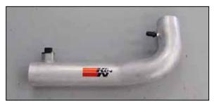
16. Install the vent fitting into the K&N® intake tube. **NOTE: Plastic NPT fittings are easy to cross** thread. Install the vent fitting "hand" tight, then turn it two complete turns with a wrench.
