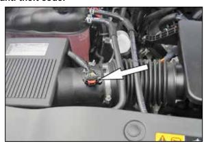
2. Disconnect the mass air sensor electrical connection and unhook the wiring harness from the air filter housing.
