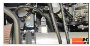
19. Reconnect the mass air sensor electrical connection.
