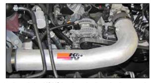
17. Install the K&N® intake tube into the hose at the filter adapter and then into the hose at the throttle body. Adjust the tube for best fit and then secure with the provided hose clamps.
