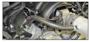
18. Install the provided crank case vent hose onto the valve cover port and onto the vent installed into the intake tube. Secure the hose with the provided hose clamps.
