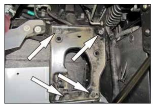
7. Remove the four bolts that secure the air filter housing mounting plate and then remove the plate from the vehicle.
