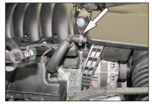
3. Disconnect the crank case vent from the intake plenum and valve cover port and remove it from the engine.
