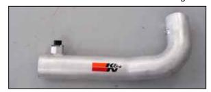
15. Install the mass air sensor assembly into the K&N® intake tube and secure with the provided hardware.
