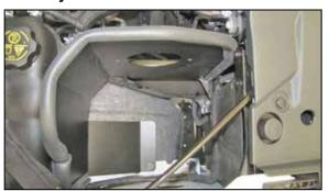
9. Install the heat shield and secure it to the air filter housing mounting plate location using three of the factory bolts from step #7.
