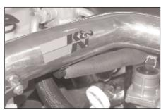
16d. Re-install the intake tube onto the vehicle, then install the 90 degree fitting into the grommet on the intake tube as shown.
