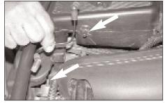
5. Remove the vacuum hose from the fuel pressure regulator and from the resonator as shown.
