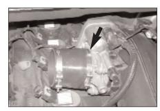
13. Install the silicone hose and hose clamps onto the throttle body as shown. The hose clamp on the throttle body may be tightened at this time.
