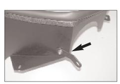
11. Install the provided bracket onto the heat shield using the provided hardware but do not tighten completely at this time.
