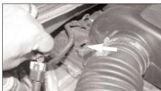
4. Unclip the air temperature sensor harness from the resonator as shown.
