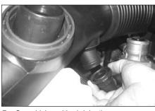
7a. On vehicles with air injection squeeze release ring then remove air injection line from intake tube.
