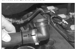
16a. On vehicles with air injection cut the vent hose 1" from end of hose.
