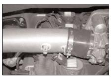
15. Slide the K&N® intake tube into the silicone hose at the throttle body as shown.
