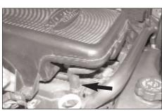
7. Loosen the hose clamp at the throttle body, then, lift the resonator upwards and disconnect the crank case vent hose as shown.
