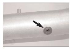
14. Install the provided grommet into the hole on the K&N® intake tube as shown.
