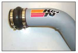
15. Install the silicone step hump hose and hose clamps onto  $K\&N^{\mbox{\tiny $\$$}}$  intake tube as shown.
