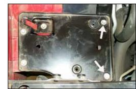
2. Remove the bolt that secures the engine cover, then, remove the engine cover as shown.
