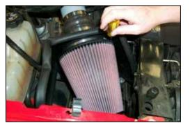
18. Install the K&N<sup>®</sup> air filter onto the mass air adapter and secure it with the provided hose clamp as shown.
