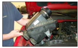
6. Pull firmly upwards to remove the air cleaner assembly as shown.
