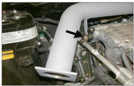
14. Line up the bracket with the stud from step 9 as shown.
