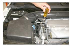
2. Remove the bolt that secures the air intake tube as shown.
