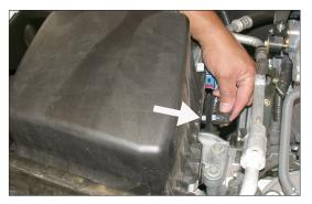
4. Disconnect the air temperature sensor electrical connection as shown.
