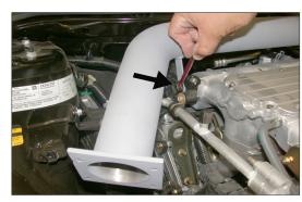
15. Secure the bracket to the stud using the nut removed in step 9 but do not tighten completely at this time
