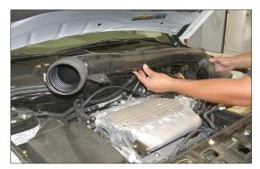
3. Loosen the hose clamps at the rubber boot on the throttle body and at the air cleaner assembly, then, remove the stock intake tube as shown.
