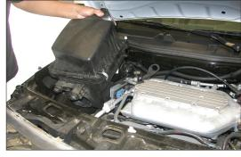
6. Pull upwards to remove the complete air cleaner assembly as shown.
