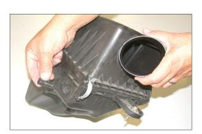
7. Remove the air temperature sensor from the air cleaner as shown.
