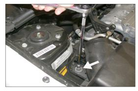
5. Loosen and remove the bolt at the back of the air cleaner as shown.
