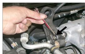
9. Remove the nut from the nylon bracket on the intake manifold as shown.
