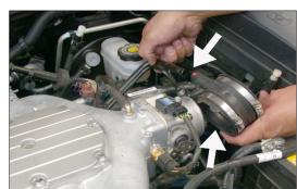
8. Remove the rubber coupler from the throttle body and disconnect the crank case vent as shown.
