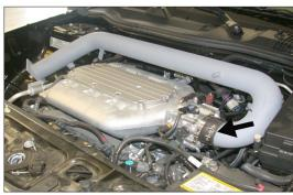
13. Install the K&N® Intake tube into the silicone hose on the throttle body as shown.
