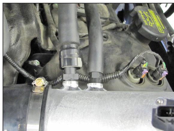
19. Connect the EVAP vent line and crank case vent lines to the fittings installed into the K&N® intake tube.
