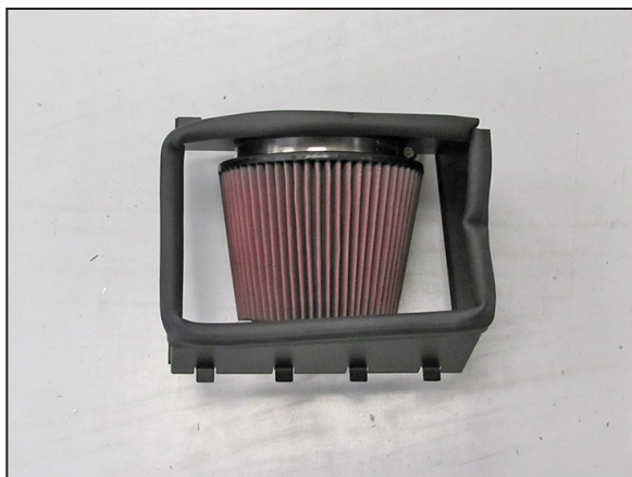
12. Install the K&N® air filter onto the filter adapter and secure with the provided hose clamp.
