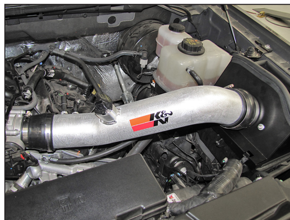
18. Install the K&N® intake tube into the silicone hose at the throttle body and then into hump hose at the filter adapter. Then secure with the provided hose clamps.
