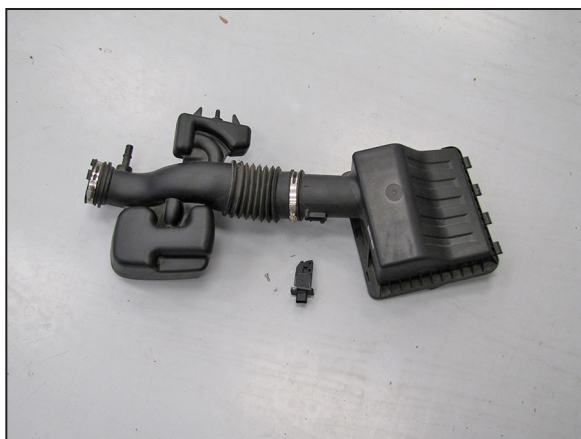
16. Remove the mass air sensor from the stock upper air box housing.
