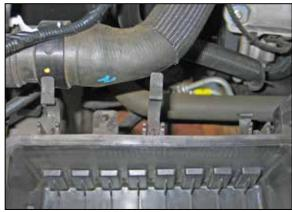
12. Remove the center upper air box retaining clip from the lower air box.
