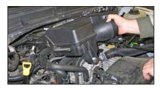
8. Unhook the heater hose clip from the intake plenum and then remove the plenum from the vehicle.
