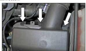
3. Release the three upper air box retaining clips.
