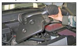
5. Remove the stock intake tube, upper air box and air filter from the vehicle.
