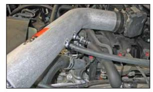
20. Connect the crank case vent hose and EVAP vent hose to the K&N® intake tube.
