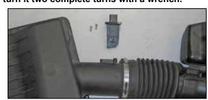
17. Remove the mass air sensor from the factory air box.
