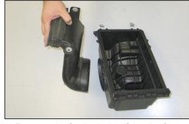
22. Remove the fresh air duct from the factory airbox.
