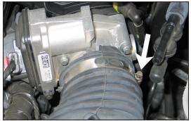
5. Loosen the hose clamp that secures the factory intake tube to the throttle body.
