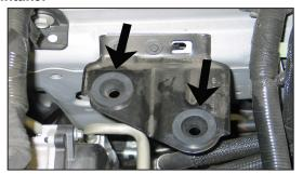
11. Remove the airbox mounting grommets shown, from the airbox mounting bracket.
