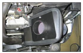
16. Set the heat shield onto the rubber mounted studs and then secure with the provided hardware. Install the K&N<sup>®</sup> air filter onto the adapter and secure with the provided hose clamp.
