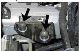
14.Install the provided rubber mounted studs onto the airbox mounting bracket as shown.
