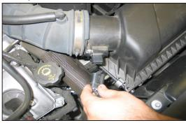
2. Release the locking tab and then disconnect the mass air sensor electrical connection.
