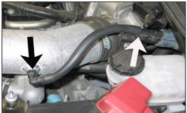
26. Attach the provided EVAP hose onto the fitting on the intake tube and then attach the open end to the EVAP check valve as shown.
