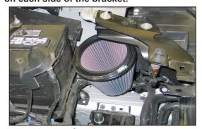
15. Set the K&N $^{\! \rm I\! R}$  air filter into the engine compartment as shown.
