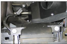
23. Install the fresh air duct into the heat shield and secure it with the factory screws in the original location, then reinstall the cover onto the core support.
