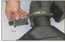
20. Remove the two screws that secure the mass air sensor to the factory airbox and then remove the sensor from the airbox as shown.
