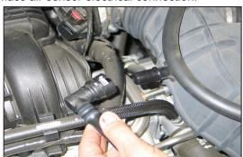
3. Release the locking tab and then disconnect crankcase vent tube from the factory intake hose as shown.
