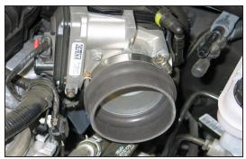
17. Install the provided silicone hump hose (084079) onto the throttle body and secure with the provided hose clamp.
