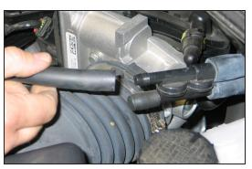
4. Disconnect the EVAP hose from the check valve as shown.
