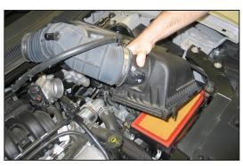
7. Disconnect the factory intake tube from the throttle body, then remove the upper airbox and intake tube from the vehicle.
