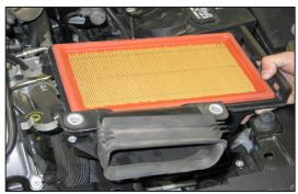
10. Lift up the lower airbox to dislodge it from the mounting grommets, then remove the lower airbox and fresh air duct from the vehicle.
