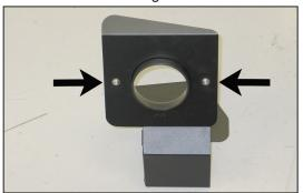
12. Install the K&N<sup>®</sup> filter adapter onto the heat shield and secure with the provided hardware.
