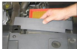
8. Remove the fresh air duct cover from the core support as shown.
