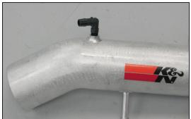
18. Install the  $90^{\circ}$  vent fitting into the intake tube as shown.
