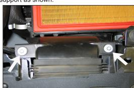
9. Remove the two bolts that secure the fresh air duct to the core support.
