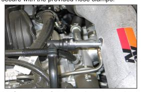
25. Connect the factory crankcase vent tube to the intake tube as shown.
