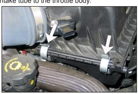
6. Release the two upper airbox latches shown.
