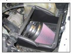
16. Place the filter assembly into the lower air box housing as shown.
