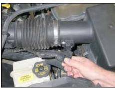
2. Release the red locking clip and then disconnect the mass air sensor electrical connection; unhook the wiring harness from the power steering reservoir.
