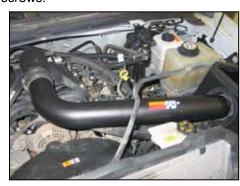
19. Place the K&N® intake tube through the heat shield, install the air filter assembly onto the end of the tube then install the intake tube into the silicone hose on the intake plenum. Secure the intake tube with the hardware and hose clamps provided.
