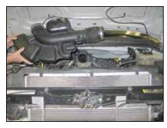
Remove the stock intake tube from the vehicle.
