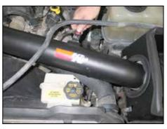
20. Connect the mass air sensor electrical connection.
