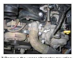
7.Remove the upper alternator mounting bolt shown.
