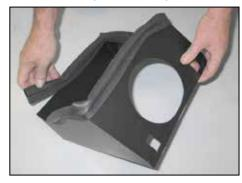
9. Install the provided long edge trim onto the heat shield as shown.
