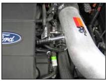
22. Connect the crank case vent hose to the  $K\&N^{\otimes}$  intake tube.
