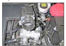
15. Install the silicone hump hose (084079) onto the throttle body and secure with the provided hose clamp.
