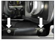
17. Feed the bottom of the fresh air scoop into the heat shield and then secure the scoop with the factory bolts removed in step #6.
