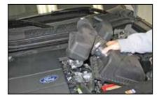
5. Release the two upper air box retaining clips and then remove the upper air box and intake tube assembly from the vehicle.
