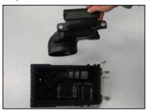
16. Remove the screw securing the fresh air intake scoop into the factory air box and pry the scoop out
