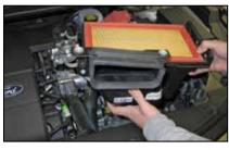
7. Remove the lower air box/fresh air duct from the vehicle.
