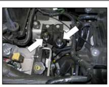
9. Install the two provided rubber mounted studs onto the air box mounting bracket as shown.
