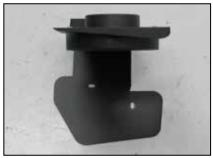
10. Install the K&N® filter adapter into the heat shield as shown and secure with the provided hardware.
