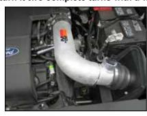
21. Install the K&N® intake tube into the silicone hose at the throttle body and then into the silicone hose on the filter adapter; secure with the provided hose clamp.
