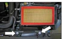
6. Remove the two fresh air duct retaining bolts shown.
