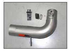
19. On vehicles that are equipped with a mass air sensor install the sensor into the K&N® intake tube and secure with the provided hardware. On all other vehicles, install the provided gasket onto the block off plate and install the block off plate into the K&N® intake tube and secure with the provided hardware.
