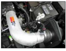
24. Connect the provided mass air sensor extension harness to the factory harness and connect the open end to the mass air sensor. Secure the mass air sensor extension harness to the vehicle wiring harness with the provided tie wrap.
