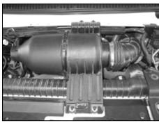
5. Remove the two bolts that secure the air filter housing to the radiator core support.
