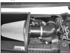
29. Insert the K&N® intake tube into the silicone hose at the throttle body and secure with the provided hose clamp.
