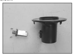
13. On 2006 models, remove the two screws that secure the mass air sensor to the housing and then remove the sensor from the housing as shown.
