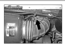
3a. On vehicles equipped with an external air temperature sensor; disconnect the temperature sensor electrical connection.
