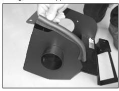
15. Install the short edge trim to the heat shield as shown. Some trimming of the edge trim may be necessary.
