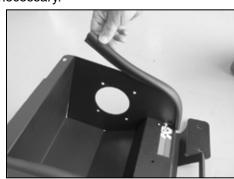
16. Install the long edge trim to the heat shield as shown. Some trimming of the edge trim may be necessary.
