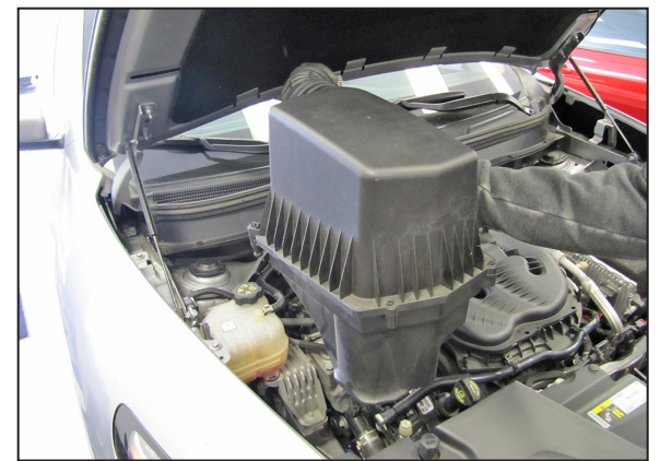
5. Lift up the air filter housing to dislodge it from the mounting grommets and then remove the complete air filter housing assembly from the vehicle. NOTE: K&N Engineering, Inc., recommends that customers do not discard factory air intake.
