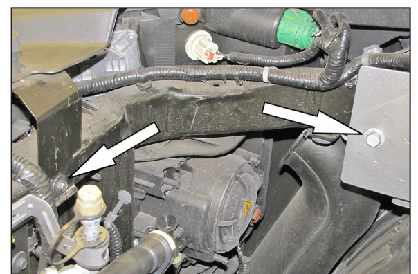
6. Remove the two factory bolts shown. NOTE: These bolts will be reused in a later step.
