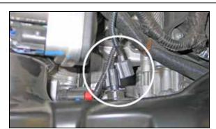
4. Disconnect the inlet air temperature air sensor electrical connection.
