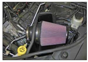
16. Install the K&N<sup>®</sup> air filter onto the adapter and secure with the provided hose clamp.
