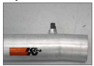
19. Install the inlet air temperature sensor into the  $K\&N^{\tiny \circledcirc}$  intake tube.
