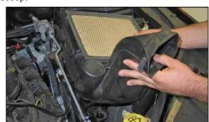
9. Lift up the lower air box to dislodge it from the mounting grommets and then remove the lower air box from the vehicle. Some vehicles may have a power steering line attached to the airbox that will need to be unhooked.
