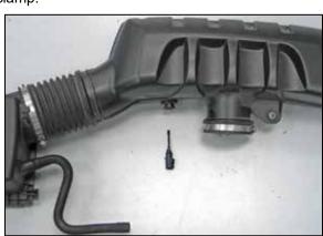
18. Release the locking tab and then remove the inlet air temperature sensor from the factory intake tube by twisting counter clockwise.
