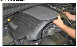
2. Lift up the engine cover to dislodge it from the mounting grommets and remove it from the vehicle
