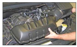
7. Remove the upper air box and intake tube assembly.
