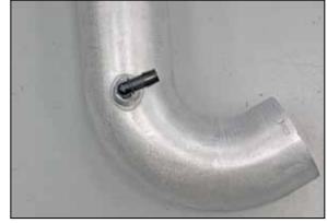
20. Install the 90° npt fitting into the K&N® intake tube as shown.
