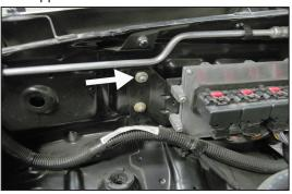
11. On 2007 model year vehicles, remove the front-upper ECU mounting nut shown.
