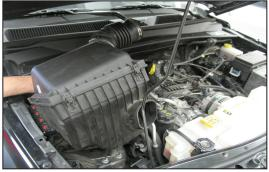
8. Pull up on the airbox assembly to dislodge it from the mounting grommets and then remove the airbox assembly from the vehicle.
