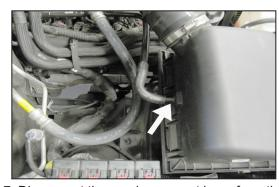
7. Disconnect the crankcase vent hose from the airbox.
