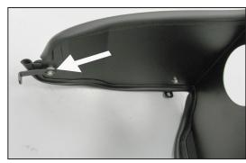
21. On 2007 and later vehicles, install the remaining small "L" bracket (06464) onto the heat shield with the provided spacer and hardware.
