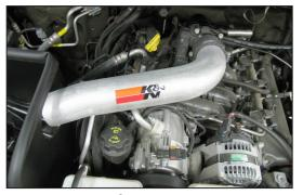
26. Install the K&N® intake tube into the silicone hose at the throttle body and align with the mounting bracket installed in step #15. Secure the tube with the hardware and hose clamp provided.
