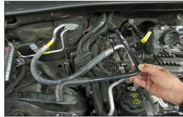
9. Unhook the crankcase vent hose from fitting on the valve cover and then remove the crankcase vent hose assembly from the vehicle.
