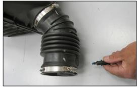
13. Remove the air temperature sensor from the stock intake tube.
