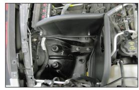
22. Install the heat shield assembly into the vehicle so that the two small "L" brackets align with the threaded stud on the inner fender and the ECU mounting stud.
