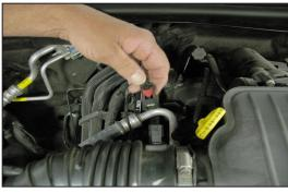
2. Release the red locking tab and then disconnect the air temperature electrical connection.
