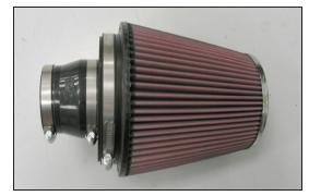
28. Install the silicone hose (08724) onto the air filter adapter and secure with the provided hose clamp.
