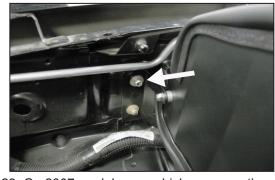
23. On 2007 model year vehicles, secure the upper heat shield mounting bracket with the nut removed in step #11.
