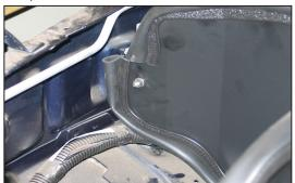
23a. On 2008 and later vehicles, secure the heat shield to the rubber mounted stud installed during step #21b.
