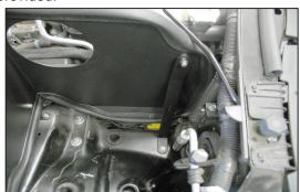
25. Secure the front heat shield mounting bracket to the inner fender with the hardware provided. NOTE: The bolt is to be installed from under the inner fender through the factory hole and bracket.
