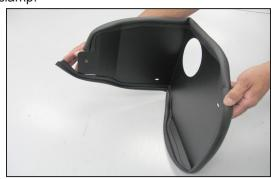
18. Install the provided edge trim onto the heat shield.
