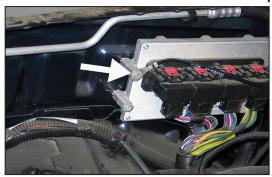
11a. On 2008 and later vehicles, remove the front-upper ECU mounting bolt shown.
