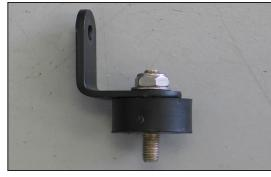
21a. On 2008 and later vehicles, attach the rubber mounted stud to the small "L" bracket (070066) with the provided hardware as shown.
