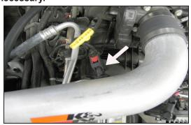
31. Reconnect the air temperature sensor electrical connection.
