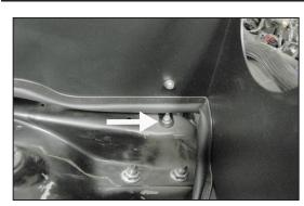
24. Secure the lower heat shield mounting bracket to the stud on the inner fender with the hardware provided.
