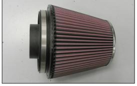
27. Install the filter adapter into the K&N  $^{\!0}$  air filter and secure with the provided hose clamp.
