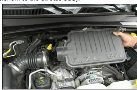
6. Remove the intake plenum from the vehicle.
