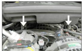
3. Remove the two "TORX" bolts that secure the intake plenum to the intake manifold with a T30 "TORX" wrench.
