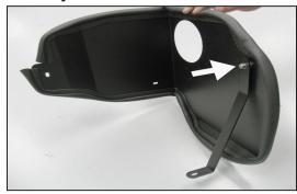
19. Install the large "L" bracket (020020) onto the heat shield and secure with the provided spacer and hardware.
