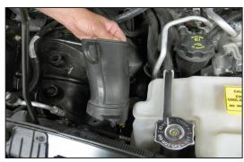
10. Remove the fresh air duct from the radiator core support as shown.
