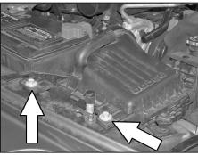
4. Remove the two airbox retaining bolts.
