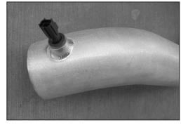
18. Install the air temperature sensor into the vent on the K&N® intake tube as shown.
