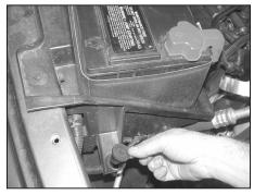
12. Install the 3/8" threaded insert provided into the airbox mounting grommet hole vacated in step #11.
