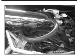
22a. On 2006 and later vehicles connect the crankcase vent hose installed in step #7c to the K&N® intake tube as shown.
