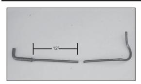
7b. On 2006 and later vehicles, measure 12" from the crankcase check valve and cut the crankcase vent tube as shown.
