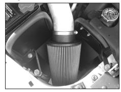
26. Install the K&N® air filter and secure with the provided hose clamp as shown.
