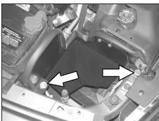
13. On the 2008 and earlier models install the K&N® heat shield assembly and secure the mounting bracket to the radiator core support with original bolt removed in step #11. Secure the rear of the heat shield to the 3/8" threaded insert with the provided hardware.
