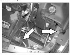
11. On 2008 and earlier models, remove the core support mounting bolt shown with a 13mm wrench, and pull out the stock airbox mounting grommet shown.
