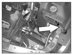
11a. On 2009 and later vehicles, the mounting bolt used has been eliminated. The heat shield bracket will need to move to the left mounting bolt which is under the radiator cover. It may be necessary to loosen the radiator cover.
