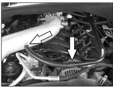
22. On 2005 and earlier vehicles connect the provided silicone hose to the crankcase vent hard line, then connect the other end to the vent on the K&N® intake tube as shown.
