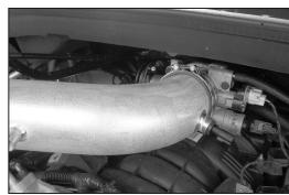
19. Slide the K&N® intake tube into the silicone hose on the throttle body as shown.
