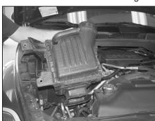
5. Pull up firmly to dislodge the airbox from mounting grommet, and remove the airbox from the vehicle.
