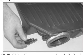
15. Twist the temp sensor counter clockwise to unlock and remove the temp sensor from the factory resonator.
