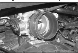
14. Install the silicone hose (084091) onto the throttle body and secure with the provided hose clamps.
