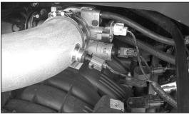
25. Reconnect the air temperature sensor electrical connection as shown.
