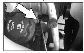
20. Line up the bracket with upper alternator mount and install the provided spacer, washer and hex bolt as shown.
