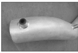
17. Install silicone hose into fitting on the K&N® intake tube as shown.
