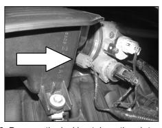
6. Depress the locking tab on the air temp sensor electrical connection and disconnect the air temp electrical connector.
