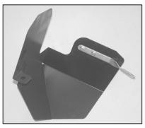
9. Install the heat shield bracket (07197) onto the heat shield with the provided hardware.
