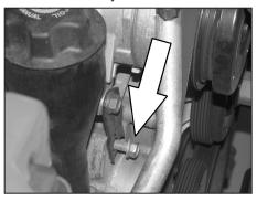
8. Remove the lower A/C bracket bolt shown with a 15mm socket.
