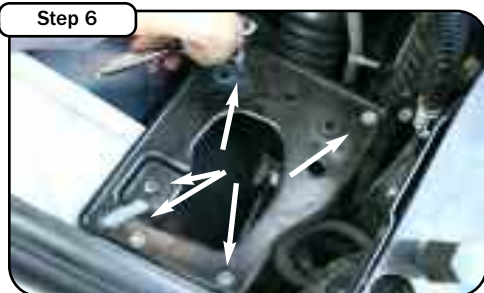
With 10mm socket, loosen the 5 screws holding the OE intake bracket and remove. Save 4 screws for later install.
