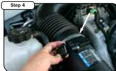
Disconnect MAF sensor harness .
