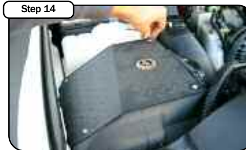
With button head screws provided, install housing cover and tighten using 5/32" allen key.
