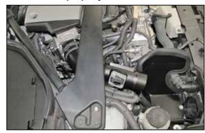
37. Install the K&N® intake tube into the coupling hose at the throttle body and align the bracket with the mounting hole in the heat shield. Adjust the tube and heat shield for proper fit and then secure with the provided hardware and hose clamp.
