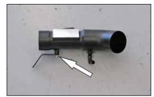
36. Install the tube mounting bracket onto the passenger side K&N® intake tube as shown and secure with the provided hardware.
