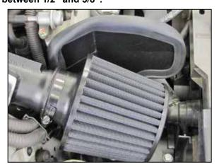
39. Install the air filter onto the intake tube and secure with the provided hose clamp.
