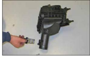
34. Remove the two screws securing the mass air sensor to the air box and then remove the mass air sensor from the air box.
