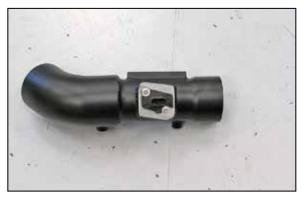
35. Install the mass air sensor into the passenger side K&N<sup>®</sup> intake tube and secure with the provided hardware.
