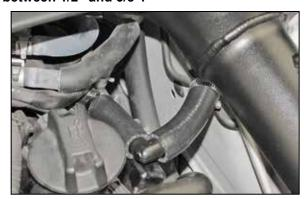
25. Connect the end of the crank case vent hose with the hose clamp to the  $90^{\circ}$  vent fitting on the driver's side K&N® intake tube and then connect the other end to the vent port on the valve cover. NOTE: Some trimming of the crank case vent hose may be necessary.
