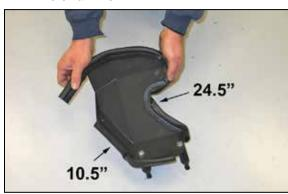
31. Install the provided edge trim onto the heat shield as shown.
