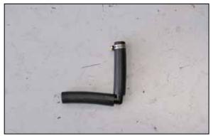
24. Connect the two 3" pieces of crank case vent hose and hose clamp to the 90° vent fitting as shown.
