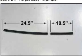
30. Cut the provided edge trim into two sections as shown. 10.5" & 24.5"
