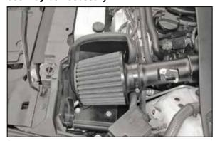
26. Install the K&N® air filter onto the K&N® intake tube and secure with the provided hose clamp.
