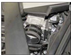
14. Install the coupling hose (084036) onto the driver's side throttle body and secure with the provided hose clamp.
