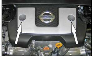
2. Remove the two bolts which secure the front engine cover and then remove the front engine cover.
