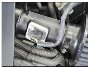
40. Reconnect the mass air sensor electrical connection.
