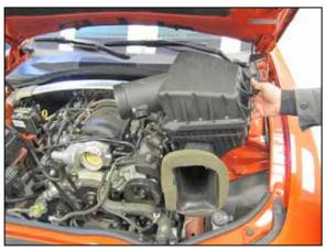
9. Lift up and remove the air box from the vehicle. NOTE: K&N Engineering, Inc., recommends that customers do not discard factory air intake.
