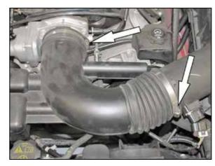
5. Loosen the hose clamps which secure the stock intake tube to the air box and throttle body.
