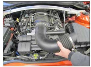
6. Remove the stock intake tube as shown.
