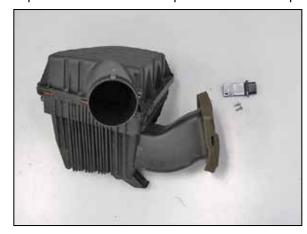
18. Remove the two screws and then remove the mass air sensor from the factory air box.
