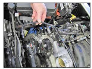
7. Rotate the crank case vent tube 180°, then release the retainer at the valve cover port and the remove the crank case vent tube.
