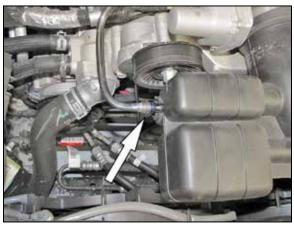
4. Disconnect the crank case vent tube from the intake resonator as shown.
