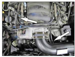
22. Attach the provided crank case vent hose to the 1/4npt fitting and then attach the open end to the vent port on the valve cover.
