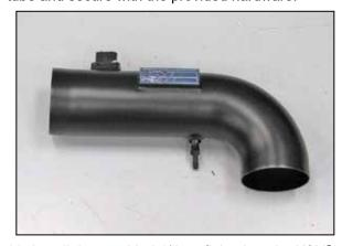
20. Install the provided 1/4npt fitting into the  $K\&N^{\circledast}$  intake tube as shown.
