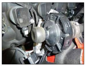
18. Install the provided cap onto the sound drum as shown.
