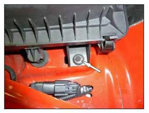
7. Remove the bolt that secures the air filter housing to the inner fender and then remove the lower air filter housing from the vehicle.
