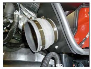
13. Install the provided hump coupler (08418) onto the filter adapter and secure with the provided hose clamp.
