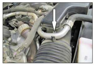
7. Unhook the coolant pipe from the intake tube.
