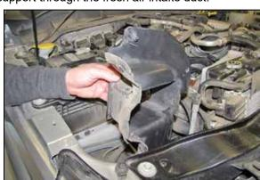
18. Remove the fresh air intake duct from the vehicle. Secure the inner fender to the vehicle with the original hardware from step #15.
