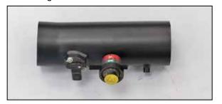
28. Install the provided grommet into the K&N® intake tube and then install the filter minder into the grommet as shown.
