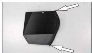
35. Install the provided edge trim onto the heat shield lid as shown.
