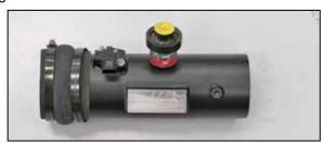
29. Install the provided silicone hump hose (08418) onto the K&N® intake tube.
