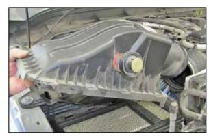
5. Remove the upper air box housing from the vehicle.
