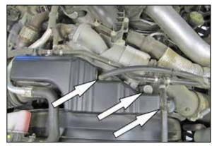
6. Unhook the coolant hoses from the intake plenum and remove the bolt securing the plenum to the engine fan shroud.
