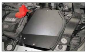
36. Install the heat shield lid onto the heat shield and secure with the provided hardware.
