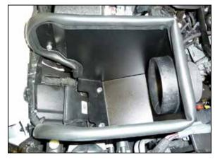
11. Install the heat shield assembly into the vehicle so that the mounting studs insert into the factory mounting grommets.
