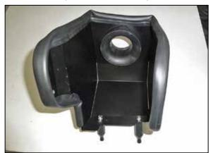
10. Install the provided edge trim onto the heat shield as shown, some trimming of the edge trim will be necessary. Install the two provided mounting studs onto the heat shield and secure with the provided hardware.
