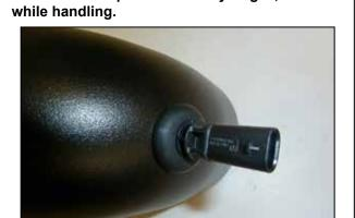
8. Install the provided grommet and factory temp sensor onto the K&N® intake tube.
