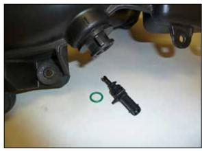
7. Remove the temp sensor from the factory intake tube by gently lifting the tab and rotating the sensor counter clockwise. Once the sensor is removed, remove the sealing O ring from the sensor. NOTE: The temp sensor is very fragile, use care
