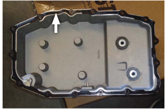
14. Inspect gasket (removed step 9) for flattened ridges or compressed edges then install it onto deep pan.
