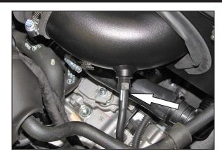
24. Connect the vacuum line to the fitting installed into the K&N® intake tube.
