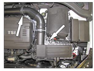
7. Release the spring clamp securing the intake tube to the turbo inlet then loosen the screw securing the air filter housing to the mount. Lift up the air filter housing to dislodge it from the mounting grommets and then remove the air filter/ hose assembly from the vehicle.
