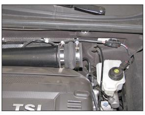
16. Install the provided coupling hump hose (08696) onto the turbo inlet and secure with the provided hose clamp.
