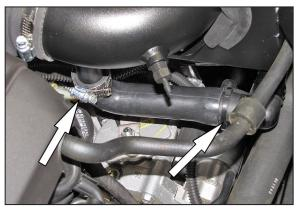
23. On vehicles that are equipped with air injection, Install the air injection hose assembly into the factory quick disconnect fitting and then install the open end onto the fitting installed on the intake tube. Secure the hose to the intake tube with the provided hose clamp. On vehicles that are not equipped with air injection, install the provided caplug onto the air injection port of the K&N® intake tube and secure with the provided hose clamp.
