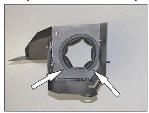
12. Install the 12.5" section into the heat shield as shown.
