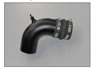
19. Install the remaining coupling hump hose (08696) onto primary  $K\&N^{\otimes}$  intake tube and secure with the provided hose clamp.
