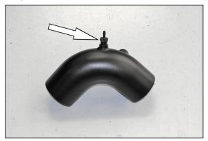
18. Install the provided vent fitting into the K&N® intake tube as shown.
