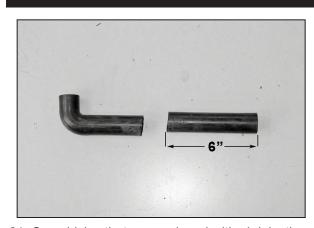
21. On vehicles that are equipped with air injection, Cut 6" off of the provided air injection hose as shown.
