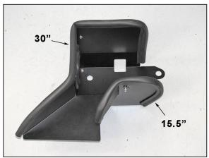
13. Install the 30" and 15.5" sections onto the heat shield as shown.
