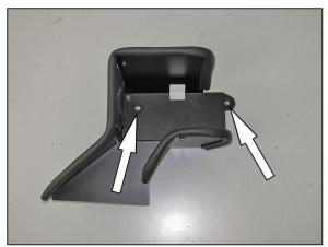
14. Install the two provided grommets into the heat shield as shown.
