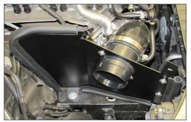
20. Set the heat shield assembly into position on the inner fender while installing the silicone hose onto the turbo inlet. Secure the heat shield with the provided hardware and secure the silicone hose with the provided hose clamps.
