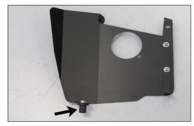
10. Install the inserted nut onto the heat shield using the provided hardware as shown.
