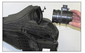
11. Remove the two screws securing the mass air
