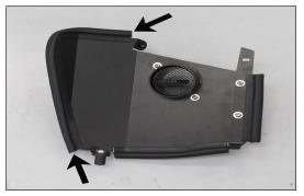
16. Install the 17" section of edge trim onto the heat shield as shown.
