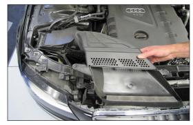
5. Unsnap the fresh air scoop from the air box and then remove the scoop from the vehicle.
