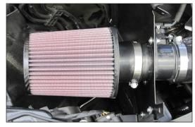
21. Install the K&N $^{\circ}$  air filter onto mass air sensor and secure with the provided hose clamp.
