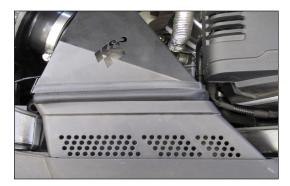
25. Reinstall the factory fresh air scoop onto the core support as shown using the factory hardware.
