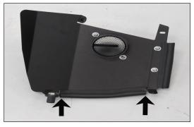
15. Install the 8" section of edge trim onto the heat shield as shown.
