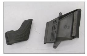
24. Separate the fresh air bellows from the fresh air scoop as shown.
