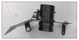
12. Install the mass air sensor into the heat shield as shown and secure with the provided hardware.
