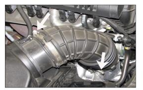
7. Loosen the two hose clamps which secure the stock intake tube to the turbo inlet and factory air box, then remove the intake tube from the vehicle.
