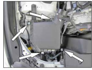
6. Release the four upper air box retaining clips and then remove the factory air filter.
