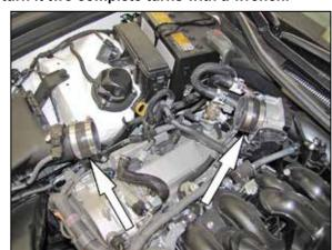
9. Install the provided coupling hoses (084031) onto the throttle body and air box as shown securing with the provided hose clamps
