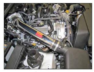
10. Install the K&N® intake tube into the hose at the throttle body and then into the hose at the upper air box. Secure the upper air box lid and then adjust the tube for best fit, secure the tube with the provided hose clamps.
