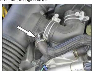
3. Release the spring clip securing the crank case breather hose to the factory intake tube and disconnect the crank case breather from the factory intake tube.
