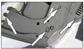
5. Remove the four clips securing the cover panel to the core support and inner fender, and then remove the panel from the vehicle.
