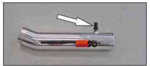
8. Install the provided vent fitting into the K&N<sup>®</sup> intake tube as shown.
