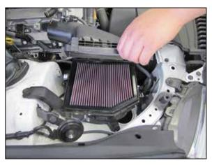
7. Install the provided K&N<sup>®</sup> air filter; do not secure the upper air box lid at this time.
