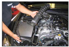
12. Remove the complete intake assembly. **NOTE: Unhook the vacuum lines clipped onto the intake tube.**
