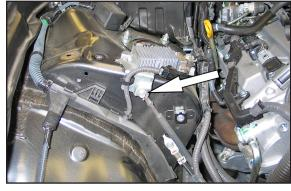
19. Remove the ground strap bolt shown.
