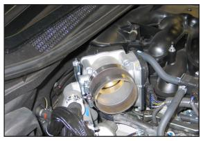
27. Install the silicone hose onto the throttle body and secure with the provided hose clamp.
