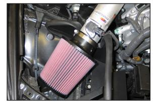
32. Install the K&N<sup>®</sup> air filter onto the intake tube and then tighten the hose clamp. NOTE: Drycharger<sup>®</sup> air filter wrap; part # RX-4990DK is available to purchase separately. To learn more about Drycharger<sup>®</sup> filter wraps or look up color availability please visit http://www.knfilters.com<sup>®</sup>.
