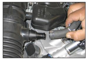
9. Unhook the crank case vent hose from the fitting in the stock intake tube.
