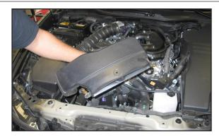
7. Remove the fresh air supply from the core support as shown.
