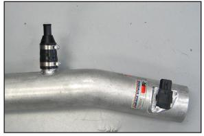
25. Install the silicone hose onto the K&N<sup>®</sup> intake tube crank case vent as shown and secure with the hose clamp, then install the factory crank case vent chamber into the silicone hose and secure with the hose clamp as shown.
