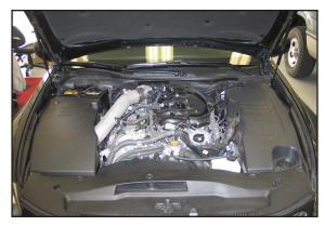
35. Reinstall the front cover and secure with the factory retainers.
