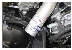
31. Using a small screw driver, remove the mass air sensor plastic elbow cover and then reconnect the mass air sensor electrical connection.
