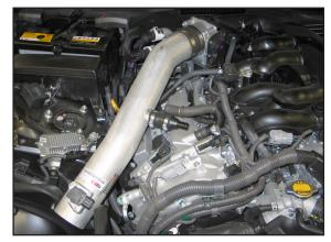
29. Install the K&N<sup>®</sup> intake tube into the silicone hose at the throttle body and align the bracket to the valve cover, secure with the factory valve cover bolt and hose clamp.
