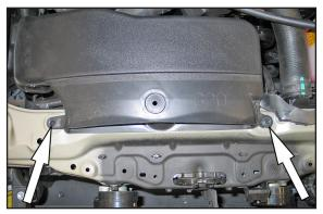
6. Remove the bolt that secures the fresh air supply to the core support.
