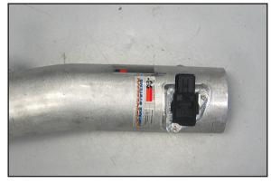
23. Install the mass air sensor into the  $K\&N^{\circledast}$  intake tube with provided bolts.
