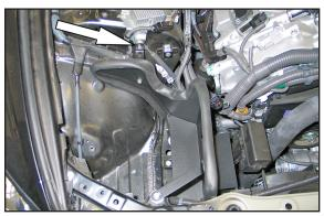
21. Set the heat shield into position and align with the rubber mounted stud, fender washer, and the ground strap bracket. Secure with provided hardware.
