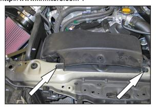
33. Reinstall the fresh air supply and secure with the factory bolt removed in step #6.
