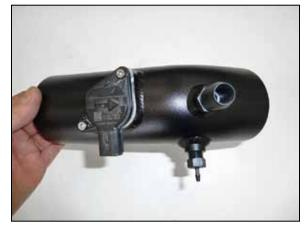
12. Remove the mass air sensor from the factory air filter housing and then install it into the K&N® intake tube and secure with the provided hardware. Install the two provided vent fittings into the K&N® intake tube as shown.
