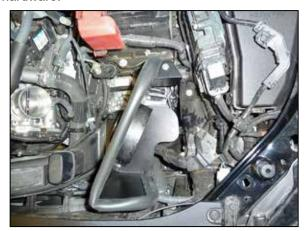
9. Install the heat shield assembly into the vehicle so that the mounting studs insert into the factory air filter housing mounting grommets
