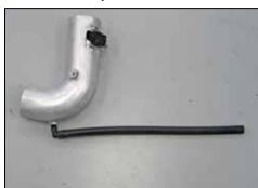
19. Install the provided crank case vent hose onto the vent fitting as shown.
