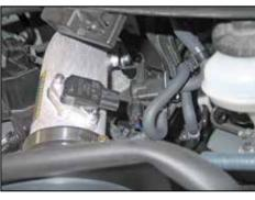
23. Secure the EVAP solenoid bracket to the intake tube with the provided hardware.
