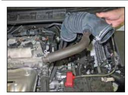
9. Release the clamp securing the intake hose to the throttle body and then remove the intake tube from the vehicle.
