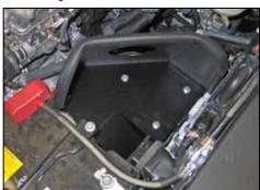
14. Install the heat shield assembly onto the rubber mounted studs, then secure the heat shield with the provided bolts and spacer.
