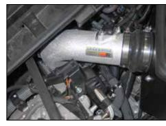
22. Install the K&N® intake tube assembly onto the throttle body and filter adapter, then secure with the provided hose clamps.
