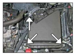
3. Loosen the hose clamp securing the intake hose to the upper air box and release the two clips securing the upper air box to the lower air box.
