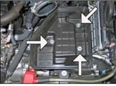
5. Remove the three bolts securing the lower air box to the mounting bracket.
