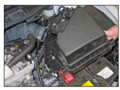
4. Remove the upper air box and air filter from the vehicle.
