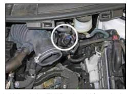
8. Unhook the EVAP solenoid from the intake tube.
