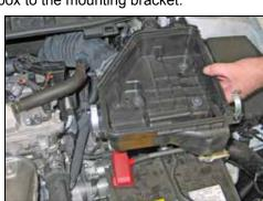
6. Unhook the fresh air duct from the lower air box, unhook the engine wiring harness from the rear of the air box and then remove the lower air box from the vehicle.
