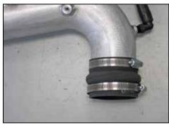
20. Install the provided silicone hose (087121) onto the throttle body end of the K&N® intake tube as shown.
