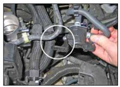
11. Install the supplied bracket (070066) onto the EVAP solenoid and secure with the provided hardware.
