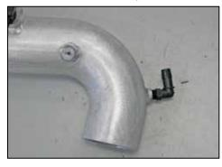
18. Install the  $90^{\circ}$  vent fitting into the K&N<sup>®</sup> intake tube as shown.
