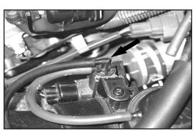
7. Disconnect the two vacuum lines from the "Vacuum switching valve."
