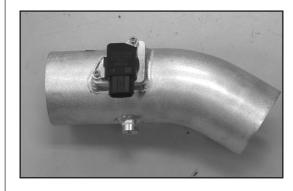
22. Install the mass air sensor removed in the previous step into the K&N<sup>®</sup> intake tube and secure with the provided hardware.
