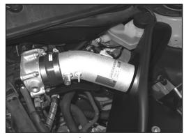
23. Install the K&N® intake tube into the silicone hose installed onto the throttle body in step # 20. Align the K&N® intake tube with the intake tube mounting bracket installed in step # 19. Secure silicone hose with provided hose clamp and mounting bracket with provided hardware.
