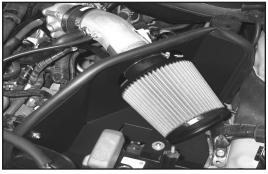
32. Install the K&N® air filter onto the K&N® intake tube; secure with the provided hose clamp.
