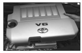
3. Gently pull the engine cover upward to release it from the mounting grommets. Once released, Remove engine cover from the vehicle and set aside.
