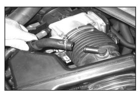
10. Release the clamp that secures the crank case vent hose to the stock intake tube and remove the crank case vent hose as shown. Loosen the clamp that secures the stock intake tube to the throttle body.
