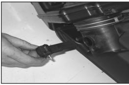
21. Remove the two screws that secure the mass air sensor to the stock intake tube. Remove the mass air sensor as shown in the photograph.
