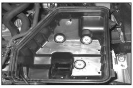
12. Remove the air filter. Remove the three bolts that secure the lower air box to the mounting bracket.
