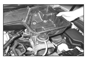
13. Remove the lower air box from the vehicle.
