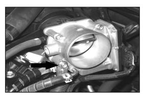
18. Remove the front lower throttle body mounting bolt.
