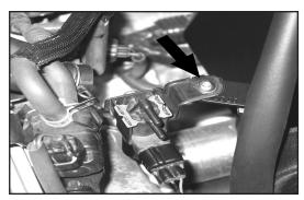
24. Secure the "vacuum switching valve" to the bracket installed onto the heat shield installed in step # 16.
