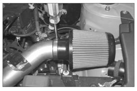
33. Install the K&N X-Stream air filter onto the K&N® Typhoon intake tube as shown.
