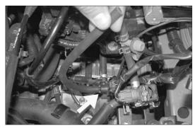
25. Install the provided silicone hose onto the EVAP OBD canister closed valve as shown.
