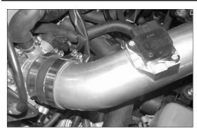
29. Slide the K&N® Typhoon intake tube into the silicone hose on the throttle body as shown. Do not tighten completely at this time.
