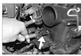
7. Disconnect the EVAP OBD canister closed valve vent hose from the air cleaner assembly as shown.
