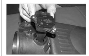
26. Remove the mass air sensor from the upper air cleaner assembly as shown.
