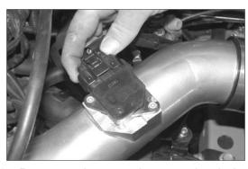
34. Reconnect the mass air sensor electrical connection as shown.
