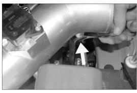
30. Line up the K&N® Typhoon® intake tube with the "C" bracket and adjust the bracket for best fit, then, secure the tube to the bracket with the provided hardware.
