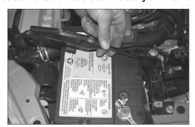
14. Remove the bolt that secures the battery hold down bracket to the radiator core support then move the bracket out of the way as shown.
