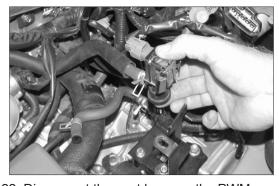
22. Disconnect the vent hose on the PWM vacuum switching valve, then, reroute the hose in front of the cruise control cable and reconnect as shown.
