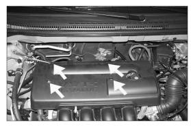
2. Using a flat blade screwdriver remove the two push clips on the engine cover as shown. Also remove the two acorn nuts on the engine cover.
