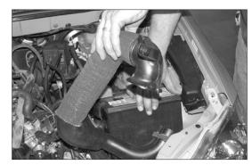
17. Tilt the battery backward and slide the air inlet duct out of the engine compartment as shown.
