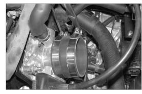
28. Install the silicone hose and hose clamps onto the throttle body and secure as shown.
