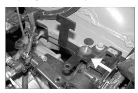
19. Secure the provided T-bracket to the stock air cleaner mount using the provided rubber mounted stud.
