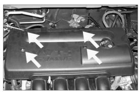
35. Reinstall the stock engine cover using the stock acorn nuts and the provided button head screws to replace the stock push clips.
