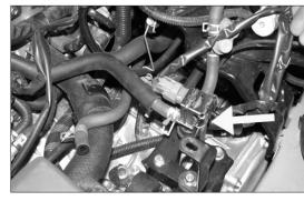
23. Slide the PWM vacuum switching valve onto the T-bracket as shown.
