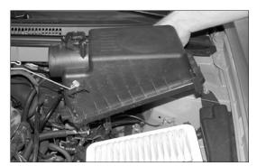
9. Remove the upper air cleaner assembly as shown.
