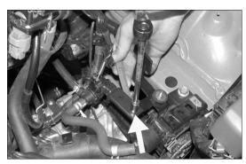
20. Secure the EVAP OBD canister closed valve to the T-bracket from step 19 using the provided hardware.
