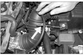
5. Remove the throttle cable from the stock wire hanger as shown.
