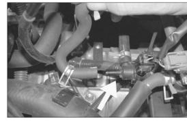
24. Remove the vent hose from the EVAP OBD canister closed valve as shown.
