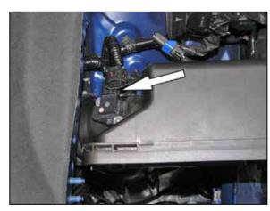
5. Disconnect the mass air sensor electrical connection.
