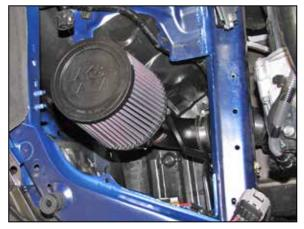
12. Install the intake tube assembly into the turbo inlet tube. Secure the tube to the mounting bracket and intake tube with the provided hardware and hose clamp.
