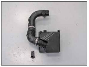
8. Remove the two screws securing the mass air sensor into the factory air filter housing and then remove the sensor.
