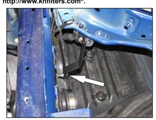
11. Install the tube mounting bracket (064327) into the factory intake tube mounting location using the provided hardware.
