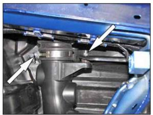
6. Loosen the hose clamp securing the intake tube and remove the nut on the lower mount.
