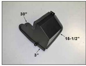
16. Install the trim onto the heat shield as shown.
