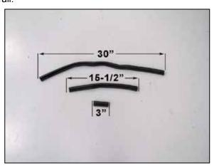
15. Cut the edge trim into three sections as shown. One section will be 30" long, one section will be 15-1/2" long and the final section will be 3" long.
