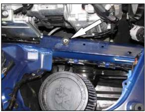
14. Install the provided rubber mounted stud into the air filter housing mounting location on the frame rail.
