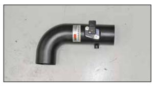
9. Install the mass air sensor into the K&N<sup>®</sup> intake tube and secure with the provided hardware.
