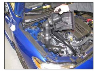
7. Separate the intake tube from the turbo inlet tube and remove the assembly from the vehicle.
