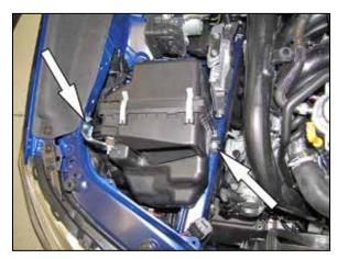
3. Remove the two nuts and one bolt securing the front half of the air filter housing to the vehicle.
