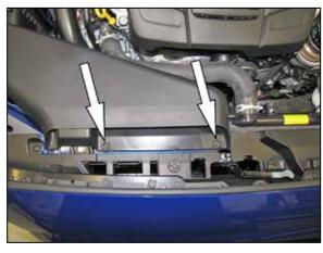
2. Remove the two clips shown securing the fresh air intake scoop and then remove the fresh air intake scoop.
