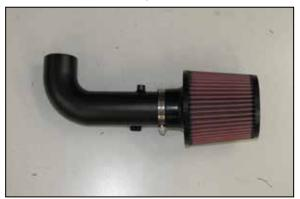
10. Install the K&N® air filter onto the K&N® intake tube and secure it with the provided hose clamp. NOTE: Drycharger® air filter wrap; part # RX-4990DK is available to purchase separately. To learn more about Drycharger® filter wraps or look up color availability please visit
