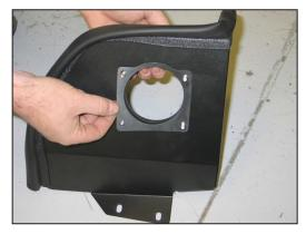
13. Install the filter adapter assembly into the heat shield and then install the remaining gasket onto the studs protruding through the heat shield as shown.
