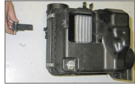
8. Remove the two screws which secure the mass air sensor and then remove the mass air sensor from the airbox as shown.
