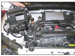
6. Remove the airbox assembly from the vehicle. NOTE: K&N Engineering, Inc., recommends that customers do not discard factory air intake.
