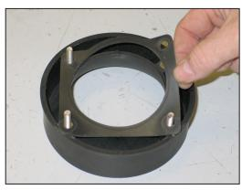
12. Install the filter adapter gasket onto the four studs as shown.
