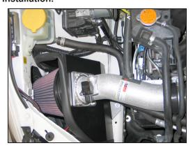
17. Install the K&N® intake kit so that the heat shield rests on the rubber mounted studs installed during step #7. Secure the heat shield with the provided hardware. Slide the silicone hose onto the turbo inlet and secure with the provided hose clamp.
