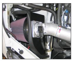
18. Reconnect the mass air sensor electrical connection as shown.
