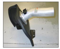
14. Install the K&N® intake tube onto the studs and secure with the provided nuts and washers.
