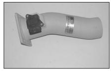
10. Install the mass air sensor into the K&N $^{\odot}$  intake tube and secure with the provided hardware as shown.
