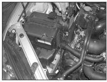
6. Loosen and remove the two hex bolts that secure the air cleaner to the inner fender as shown.
