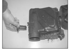
3. Remove the air inlet scoop, which is secured to the radiator core support by two plastic rivets.
