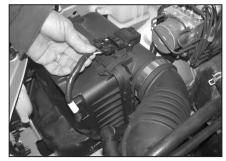
4. Disconnect the mass air sensor electrical connection and unclip the harness from the side of the air cleaner as shown.
