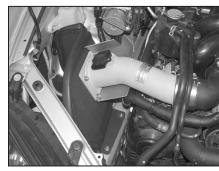
21. Line up the heat shield with the rubber mounted studs and secure with the provided nylock nuts, then, slide the intake tube into the silicone hose and secure as shown.
