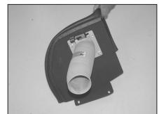
15. Install the intake tube onto the studs and secure with two of the provided nylock nuts and flat washers as shown in the orientaion.
