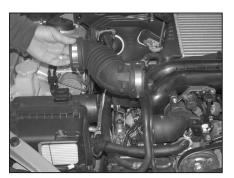
5. Loosen the hose clamps at the air cleaner and at the turbo inlet tube, then, unclip the coolants hoses from the stock intake hose and remove the stock intake hose as shown.
