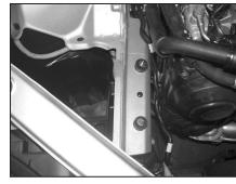
18. Install the provided rubber mounted studs into the original air cleaner mounting holes as shown.
