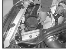
19. Place the K&N $^{\ensuremath{\circledast}}$  air filter into the cavity in the inner fender as shown.
