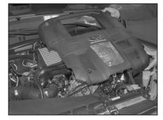
2. Remove the engine cover, which is secured by four plastic rivets.
