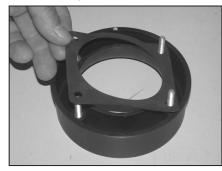
13. Apply one of the provided gaskets onto the adapter as shown.
