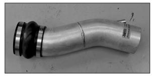
17. Install the silicone hump hose onto the intake tube as shown and secure with the provided hose clamp as shown.
