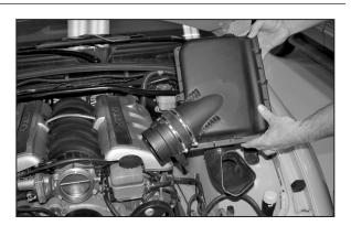
7. Pull up on the air box assembly to dislodge it from the three mounting pins and then remove the air box from the vehicle as shown.
