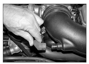
4. Disconnect the crank case vent hose from the factory intkae tube as shown.
