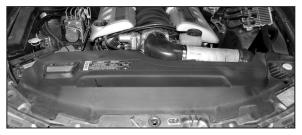
20. Reinstall the radiator cover and the five mounting clips removed in step #2.
