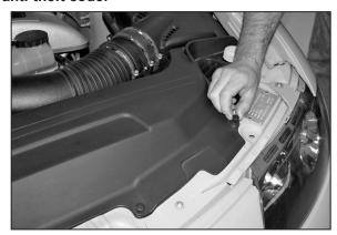
2. Release the center pin on the five radiator cover clips, Then remove the clips from the radiator cover.
