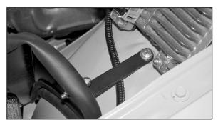
15. Install the heat shield mounting bracket onto the heat shield as shown and then secure the bracket to the inner fender at the upper air box mounting pin location as shown with the provided hardware.
