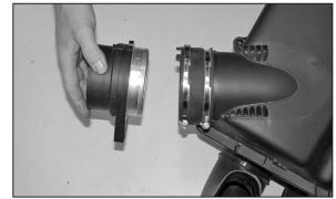
9. Loosen the hose clamp that secure the mass air sensor to the factory air box, then remove the mass air sensor from the factory air box.
