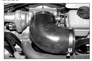
16. Install the 90° silicone hose onto the throttle body and secure with the provided hose clamp as shown.
