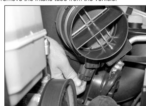
Release the mass air sensor electrical connection clip, then disconnect the electrical connection.
