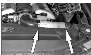
18. Install the K&N® intake tube into the 90 degree silicone hose at the throttle body and mass air sensor and secure with the provided hose clamps as shown.
