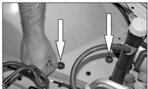
12. Place the two rubber washers onto the inner fender at the lower air box mounting pin locations as shown.
