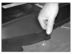
33. Reinstall the five radiator cover retaining clips removed in step #2.
