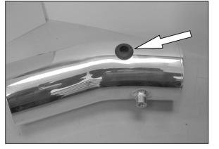
15. Install the provided rubber grommet into the K&N® intake tube as shown.
