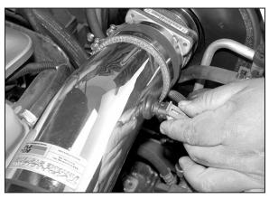
31. Reconnect the temperature sensor electrical connection.
