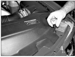
2. Release the center pin on the five radiator cover clips. Then remove the clips from the radiator cover.
