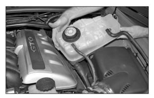
7. Pull the coolant reservoir up and away from the inner fender to release it from the retaining studs.
