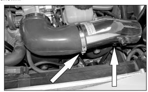
17. Install the K&N® intake tube onto the throttle body silicone hose and tighten hose clamp but not completely. Align the bracket installed in step #12 to the bung on the intake tube and tighten using the hardware provided.
