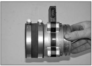
27. Install the silicone hose (#08698) onto the intake tube side of the mass air sensor and secure with the provided hose clamp.
