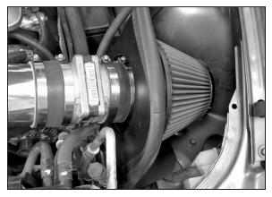
29. Install the filter charger assembly onto the K&N® intake tube and secure with the provided hose clamp.
