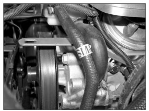
12. Install the tube bracket #010076 using the provided hardware.
