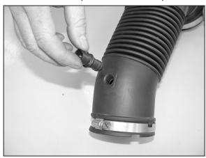
14. Remove the air temperature sensor from the stock intake tube.
