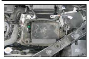
7. Remove the positive battery cable and battery mounting bracket, then remove the battery from the vehicle.
