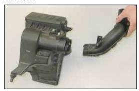
32. Remove the lower fresh air duct from the air box as shown.
