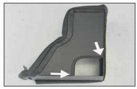
21. Install the provided edge trim into the heat shield fresh air duct opening as shown.
