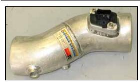
25. Install the mass air sensor into the K&N® intake tube and secure with the provided hardware.
