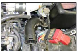
33. Install the lower fresh air duct into the heat shield as shown.
