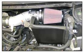
30. Install the K&N® air filter onto the intake tube and secure with the provided hose clamp.
