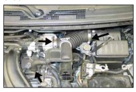
8. Loosen the two hose clamps securing the intake tube and the spring clamp securing the crank case vent hose to the valve cover.
