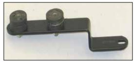
17. Install the two provided rubber mounted studs onto the heat shield mounting bracket (083125) as shown. Do not completely tighten at this time.
