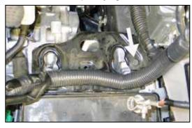
18.Remove the air box mounting plate bolt shown. **NOTE: This bolt will be reused in the next step.**
