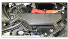
36. Reinstall the intake resonator onto the fresh air intake duct.
