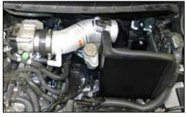
28. Install the K&N® intake tube into the silicone hose at the throttle body and align with the tube mounting bracket. Secure the intake tube with the hose clamp and hardware provided.
