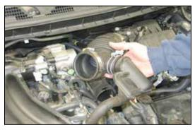
9. Remove the intake hose assembly.
