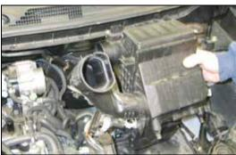
11.Lift up the air box to dislodge it from the mounting grommets and then remove the air box from the vehicle.
