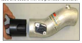
26. Install the mass air sensor venturi into the K&N® intake tube as shown.
