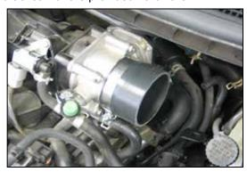
23. Install the provided silicone hose (08440) onto the throttle body and secure with the provided hose clamp.
