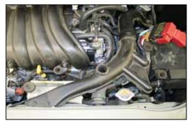
34. Install the upper fresh air duct into the lower section and then secure with the factory retaining clips to the radiator core support.
