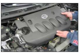
3. Remove the two bolts which secure the engine cover then remove the engine cover as shown.
