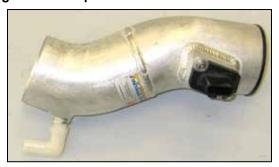
27. Install the provided 90° vent fitting onto the K&N® intake tube as shown.
