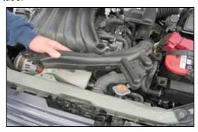
6. Remove the upper fresh air inlet duct from the vehicle.
