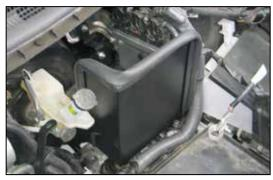
22. Set the heat shield into position on the mounting bracket and rubber mounted studs then adjust as necessary. Secure the heat shield and bracket with the provided hardware.
