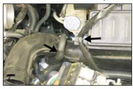
10. Disconnect the transmission vent line and wiring harness from the air box.
