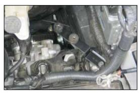
19. Install the heat shield mounting bracket assembly onto the air box mounting plate as shown and secure with the bolt from the previous step.
