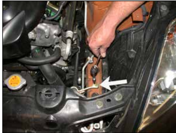
14. Remove the bolt that secures the air conditioner hard line bracket to the inner fender as shown.
