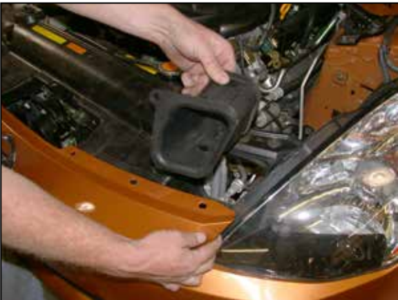
10. Pull the bumper cover forward and remove the air inlet duct as shown.
