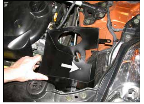
17. Install the K&N® air box into the vehicle and line up the mounting tab with the original hanger, then line up the lower mounting hole with the rubber mounted stud from step 16.
