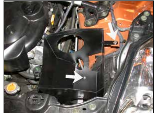
19. Reinstall the air box and secure it using the provided hardware as shown.
