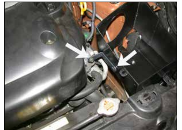
20. Using the bolt removed in step 11, secure the provided "L" bracket to the timing chain cover, then, secure the long leg of the bracket to the airbox using the provided hardware as shown.
