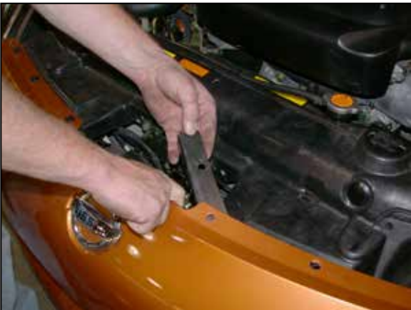
9. Loosen and remove the hex bolt that secures the Bumper cover bracket to the core support, then remove the bracket as shown.
