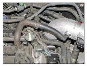
26. Connect the factory crank case vent hose to the hose mender and secure with the factory clamp.
