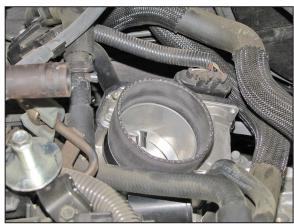
10. Install the coupling hose (084036) onto the throttle body and secure with the provided hose clamp.
