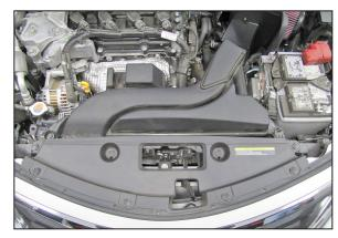
30. Install the core support cover and secure with the factory pins.
