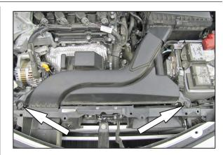
5. Remove the two bolts securing the fresh air intake to the core support and then remove the fresh air intake.
