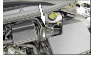
6. Loosen the hose clamp securing the intake hose to the air filter housing.
