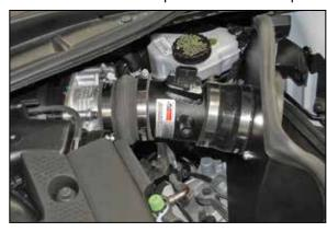
19. Install the K&N® intake tube into the hump hose, Pull the heat shield forward and install the intake tube into the hose at the filter adapter. Adjust the tube for best fit and then secure the tube with the provided hose clamps.
