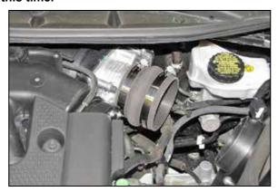
15. Install the provided hump hose (08171) onto the throttle body and secure with provided hose clamp.
