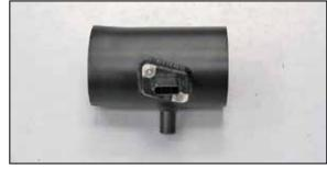
18. Install the mass air sensor into the K&N<sup>®</sup> intake tube and secure with the provided hose clamp.
