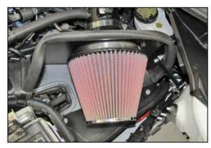
23. Install the K&N® air filter onto the filter adapter and secure with the provided hose clamp. NOTE: Drycharger® air filter wrap; part # RF-1048DK is available to purchase separately. To learn more about Drycharger® filter wraps or look up color availability please visit http://www.knfilters.com®.
