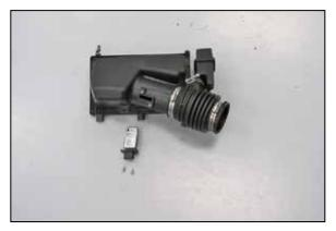
17. Remove the mass air sensor from factory air box.
