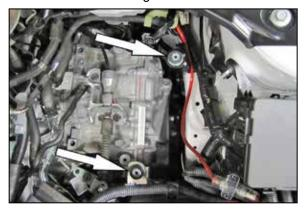
8. Install the two provided rubber mounting studs onto the air box mounting brackets as shown.
