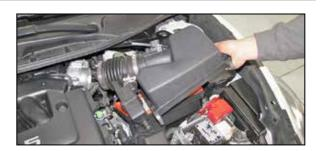
5. Release the two upper air box retaining clips and then remove the upper air box assembly.
