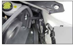
20. Secure the heat shield mounting bracket to the air box bracket on the strut tower with the provided hardware.
