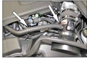
22. Install the crank case vent hose onto the fitting on the K&N<sup>®</sup> intake tube and the install the hose mender into the factory crank case vent hose and secure with the factory spring clamp.
