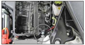
6. Remove the bolt which secures the lower air box to the mounting bracket. Remove the lower air box from the vehicle.
