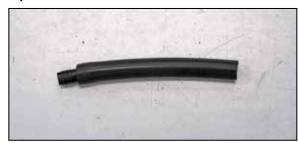
21. Install the hose mender into the provided crank case vent hose as shown.
