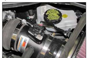
24. Reconnect the mass air sensor electrical connection.
