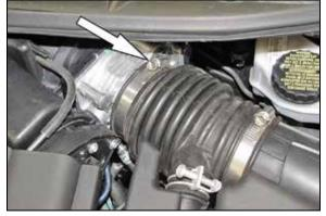
3. Loosen the hose clamp which secures the intake hose to the throttle body.
